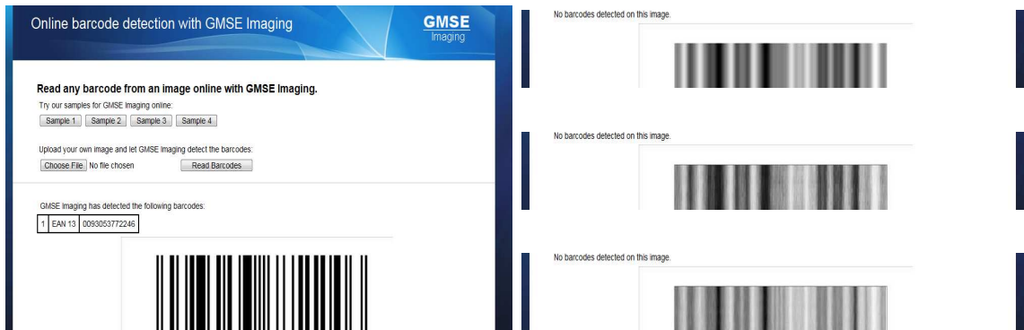
Figure 5.10: Detection results using the commercial software, GMSE imaging [72], for the idealised (left) and full-size barcode images in synthetic experiment 5.4.1 (first right) and real experiments 5.4.2 (middle right) and 5.4.3 (bottom right).
