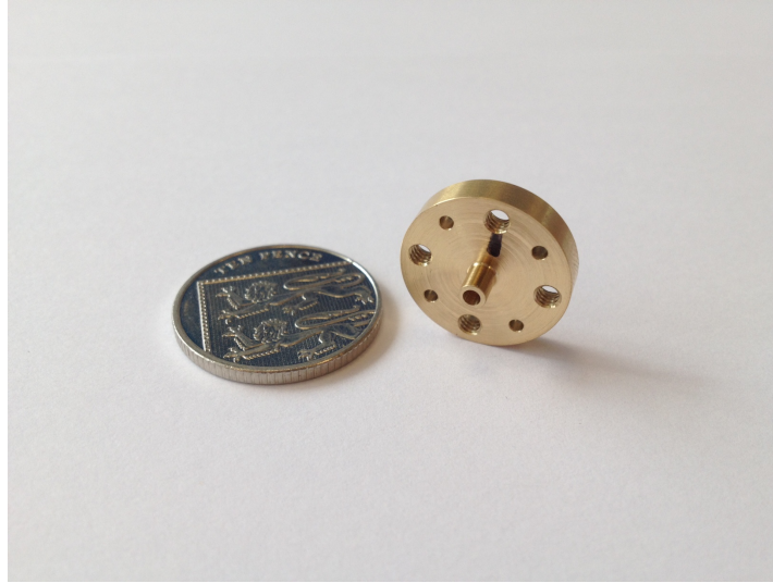
Figure 3.14: A complete, smooth-walled brass feed horn shown alongside a coin for scale.
