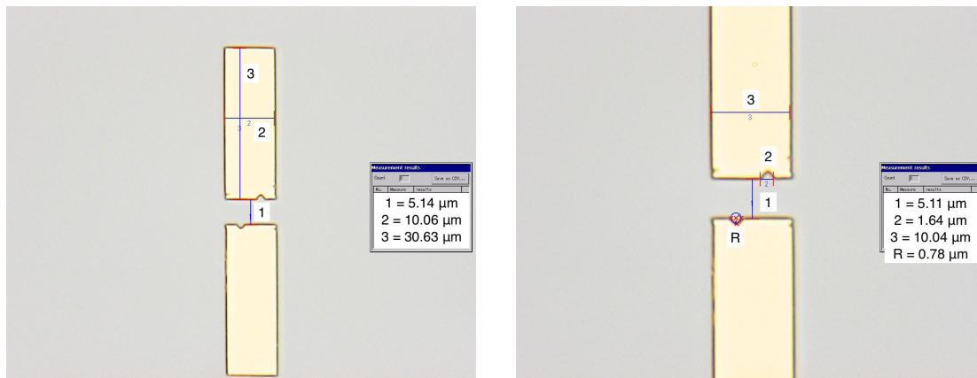
(a) Measured results under 3000 \times magnification. The dimensions of the metallised pads match the specifications and exhibit very good definition as can be seen by the straight lines and sharp corners.
