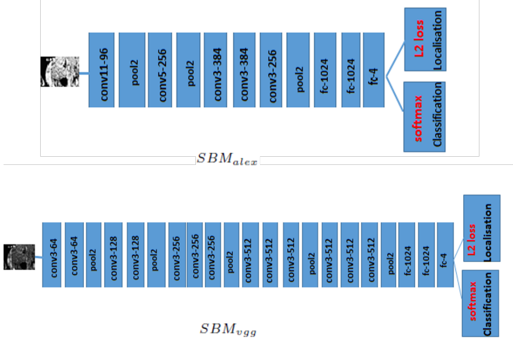
Figure 3.2: Spatial baseline models based on AlexNet ( SBM_{alex} ) and VGGnet ( SBM_{vgg} ).
