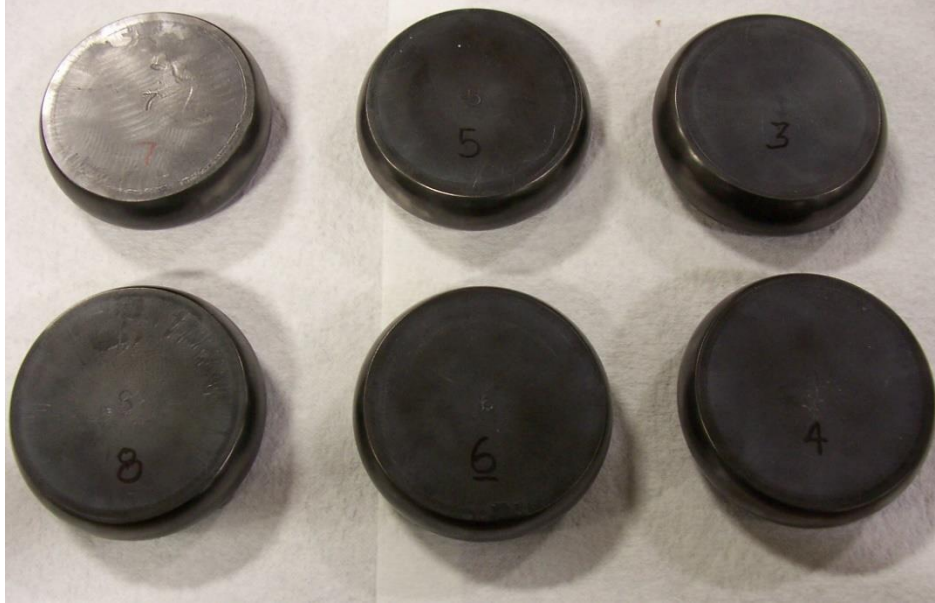
Figure 3.1 – Final pancake forgings created for the previous generation of ABD alloys (ABD-1:3). They measure approximately 110mm in diameter. Reproduced from [74] with permission from the copyright holder D Crudden © 2014.
