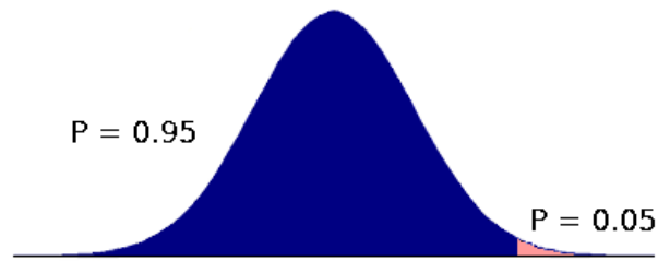
Figure 4.1: The probability-distribution for a t-test. The samples' difference in means, the samples' standard deviation, and the samples' sizes are used to calculate the t-statistics. Using a table of critical values, the probability p , i.e. the probability that the given distribution would generate a sample that has a t-score of t or beyond, can be calculated. If there is a significant difference (the probability for this is marked in red), then it is likely that the two samples come from two populations that differ in means.
