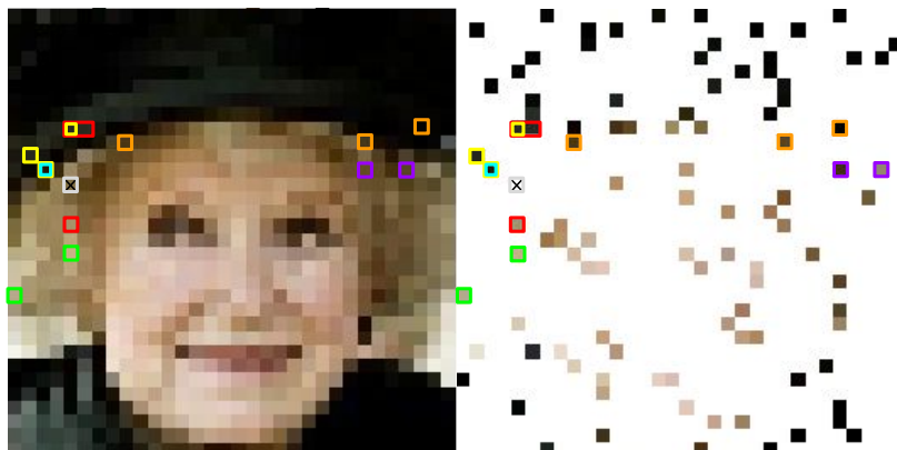
Figure 6.16: Visualisation of pixels attended by each head of multihead attention in the NP given a target pixel and a separate context of 100 random pixels. Each head is given a different colour (consistent with the colours in Figure 6.6 and the target pixel is marked by a cross).
