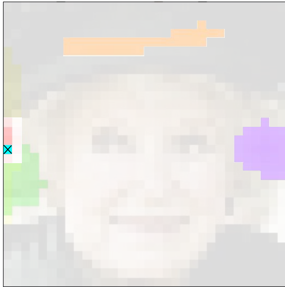
Figure 6.6: Pixels attended to by each head of multihead attention in Multihead ANP given a target pixel. Each head is given a different colour and the target pixel is marked with a cross.
