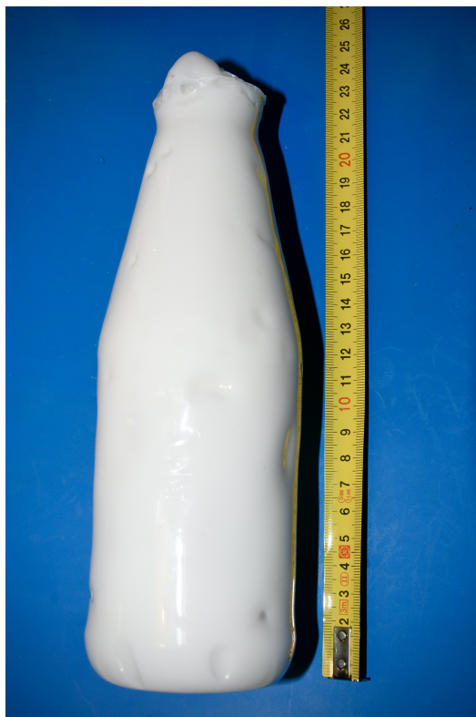
Figure 2. Sample 22 cm high, obtained starting from 600 g of MMA, loaded with 2% w of Gd (equal to 2.3% w Gd 2 O 3 ).
