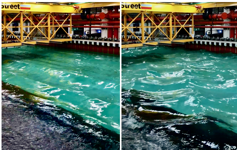
Figure 1.2: An operating 12 × 20 m wave flume with waves generated by multiple paddles (in red) and absorbed by the wave absorber (in dark-blue) at the bottom-left of each image). Unidirectional waves are generated by paddles which are moving in phase; cross waves are generated by imposing constant phase shifts between consecutive paddles. Images are taken at the Hydrodynamics laboratory, Imperial College London.
