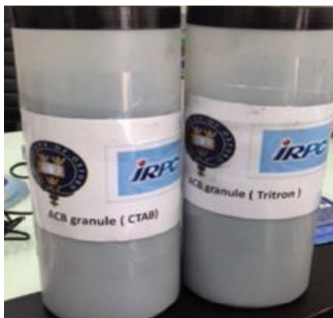
Figure 7.1: Processed ACB and Triton X-100 modified ACB by the granulation method at 500g scale.
