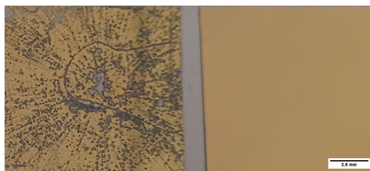
Figure 7.13: Images of gold thin film electrodes on PET substrates. Left) Prepared by UV/O 3 -PDMS stamped deposition, Right) Prepared by thermal evaporation through a shadow mask.
