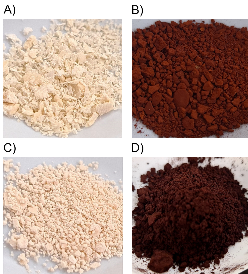
Figure 4.30: Images of A) N-succinimidyl 3-thiophene acetate (S3TA), B) P(3HT-c-S3TA) (13), C) N-succinimidyl 3-(thiophen-3-yl)acrylate (S3T3YA), and D) P(3HT-c-S3T3YA) (14).
