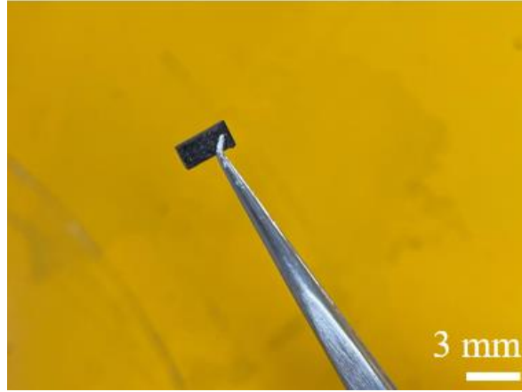
Figure 4.5 An example of an MgB_2 piece cut for magnetisation measurement.
