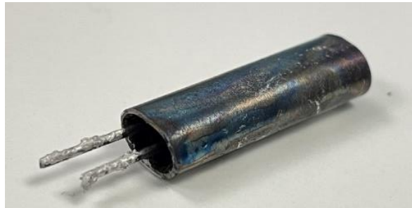
Figure 6.13 The short joint comprises reacted wires encased within a titanium tube filled with a mixture of Mg and B (stoichiometric ratio of 1:2) powder.
