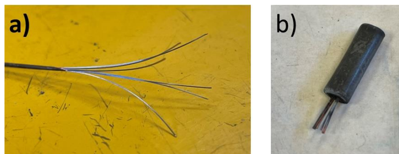
Figure 7.7 a) Etched MgB 2 multifilament, and b) short joint made using the etched wire.
