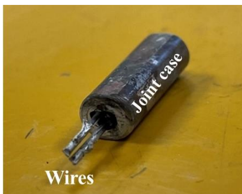
Figure 6.6 One of the short joint example. The wires, each measuring 2 cm in length, were placed into two holes, each 1 cm deep, drilled into the compressed Mg+B powder contained within the case.
