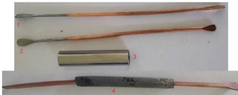
Figure 2.25 MgB 2 joint design by groove-rolling process reprinted from [193] (Copyright © 2016, IEEE). As a scale reference, the wire diameter is 1.6 mm.
