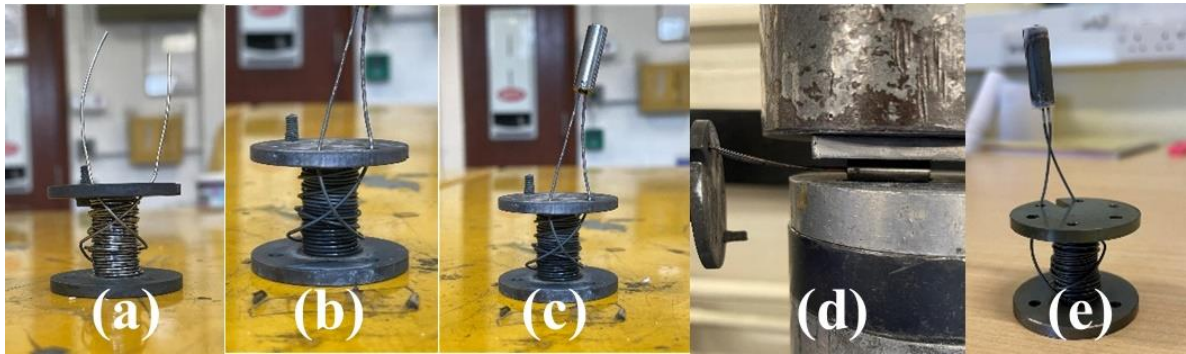
Figure 6.1 MgB 2 coil making steps. a) MgB 2 coil before the initial heat treatment (700 °C for 15 minutes), b) after heat treatment, c) joining the wire tips, d) mechanical pressing of the joint e) after heat treatment (900 °C for 30 minutes and 650 °C for 1 hour) of the joint.
