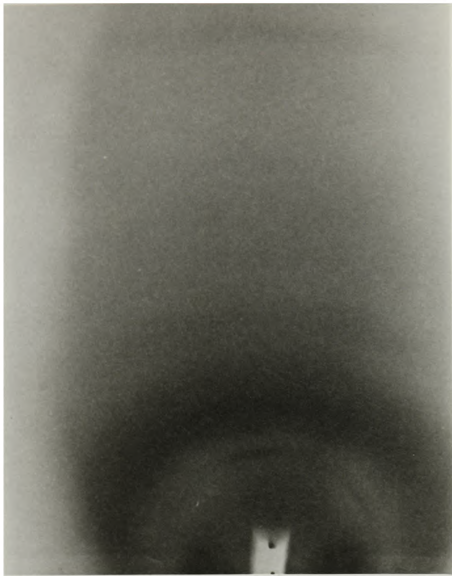
Plate 5.8 X-ray diffraction pattern taken at room conditions of fibres drawn from the left colleterial gland of S.membranacea . The fibres are tilted by 31° to show the 1.49Å reflection. 7 day exposure.
