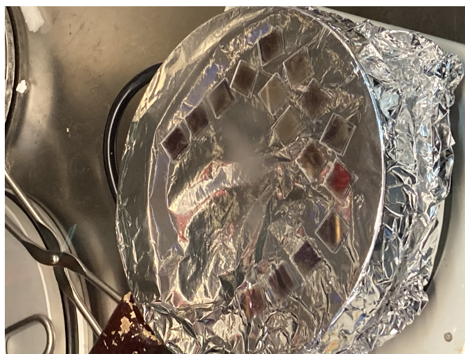
Figure 5.3: Photograph of film substrates in the process of being post-annealed at 140 °C. Samples appear to be partially changing colour from purple to grey.
