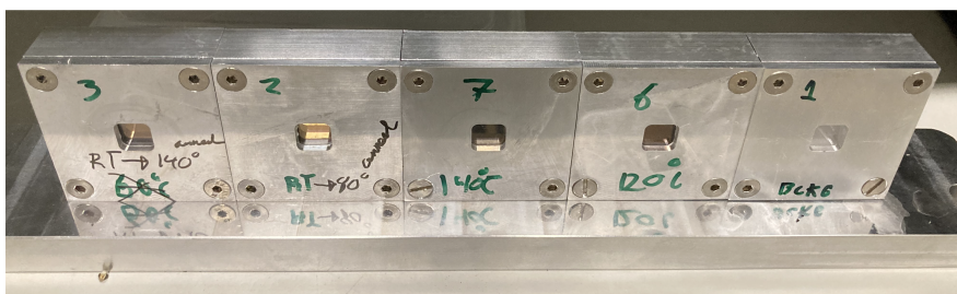
Figure 5.5: Five neutron holders mounted on the changing rack.
