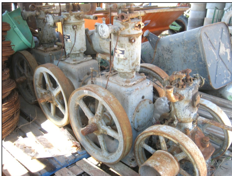
Photograph 6.2 Dieter engines for noria in Manzanares
