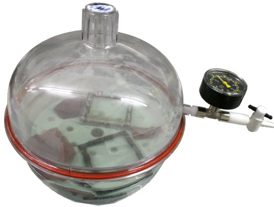
Figure 3.6: Degassing setup for ox liver. A desiccating chamber is used to set up an enclosed environment in which a partial vacuum of -0.9 bar can be created using a vacuum pump. Once the pressure is attained, the valve at the right can be switched off. Pressure can be monitored using the meter next to the valve. To ensure no air enters the inside of the tissue holder, both tissue and holder are degassed under phosphate buffered saline solution for 30 mins before being assembled in the solution.
