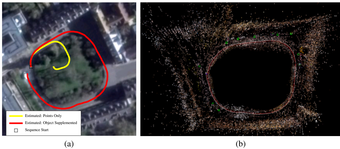
Figure 2.21: (a) Resultant trajectories estimated using point-only bundle adjustment (yellow), and object-supplemented bundle adjustment (red). Satellite imagery of the mapped area is shown for comparison. Satellite imagery: Google, DigitalGlobe. (b) Point cloud from video sequence with varying height. Objects are shown in green.
