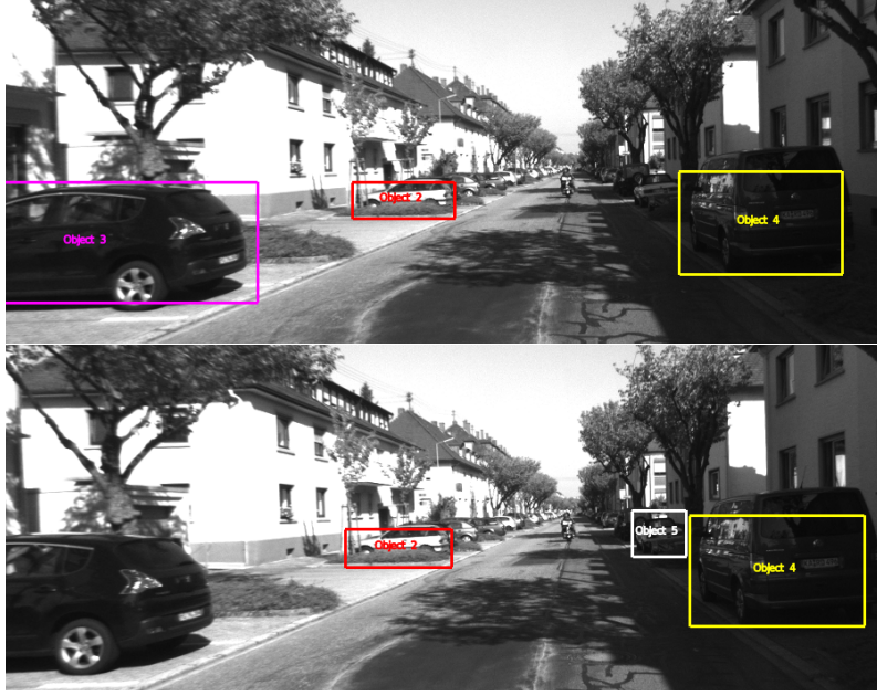
Figure 2.8: Object detections from two adjacent keyframes. Detections and their associated labels act as measurements for objects.
