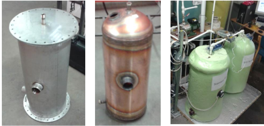
Figure 4-1 (Left) photograph of the stainless and (centre) copper test tanks prior to insulation (right)
