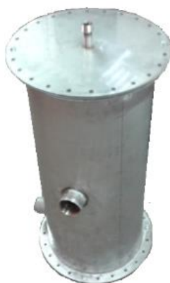
Figure 5-15 Stainless steel test tank before insulation was applied
