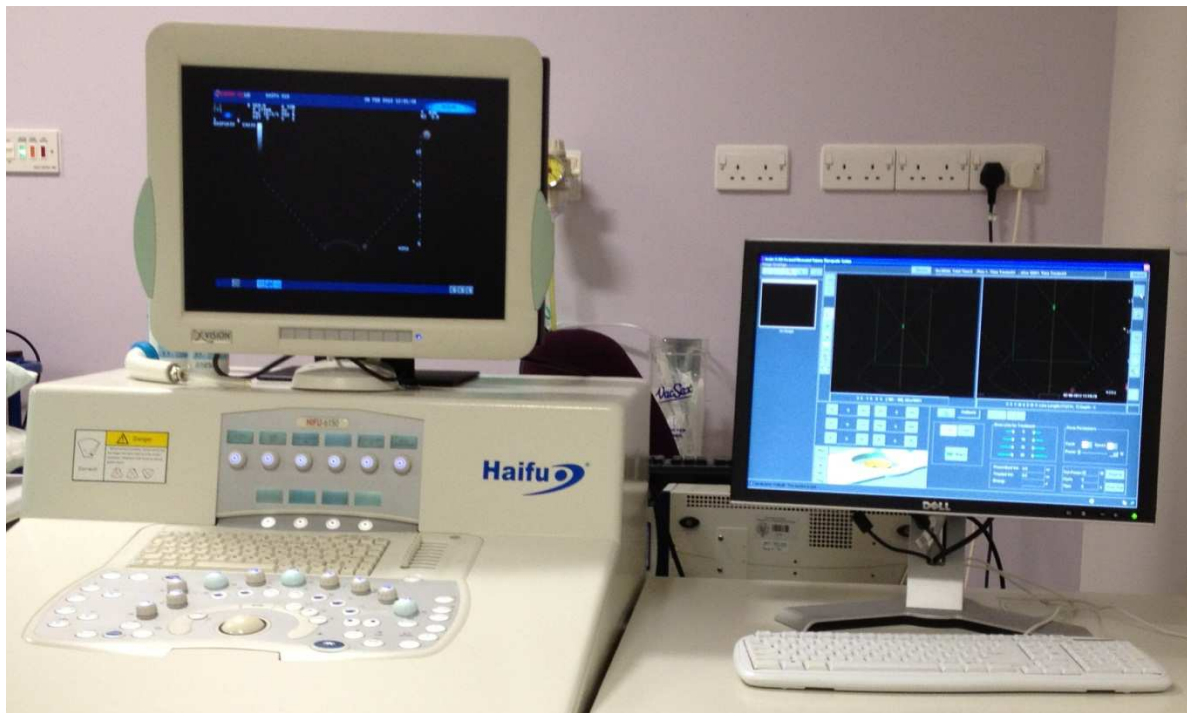
Figure 17 – Photograph of operator console from JC200 HIFU device. The left screen displays the diagnostic image from the integrated diagnostic ultrasound probe within the treatment head. The right screen display the operator console to control the degassing, water reservoir and HIFU output functions.
