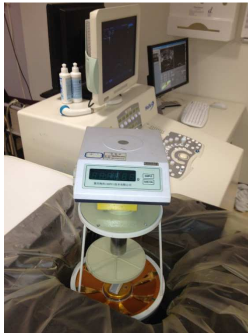
Figure 72 – Photograph of RFB positioned over transducer with mount and sub-array in place. Radiation force measurements were taken at 50-450W output in 50W steps (3 measurements at each output)
