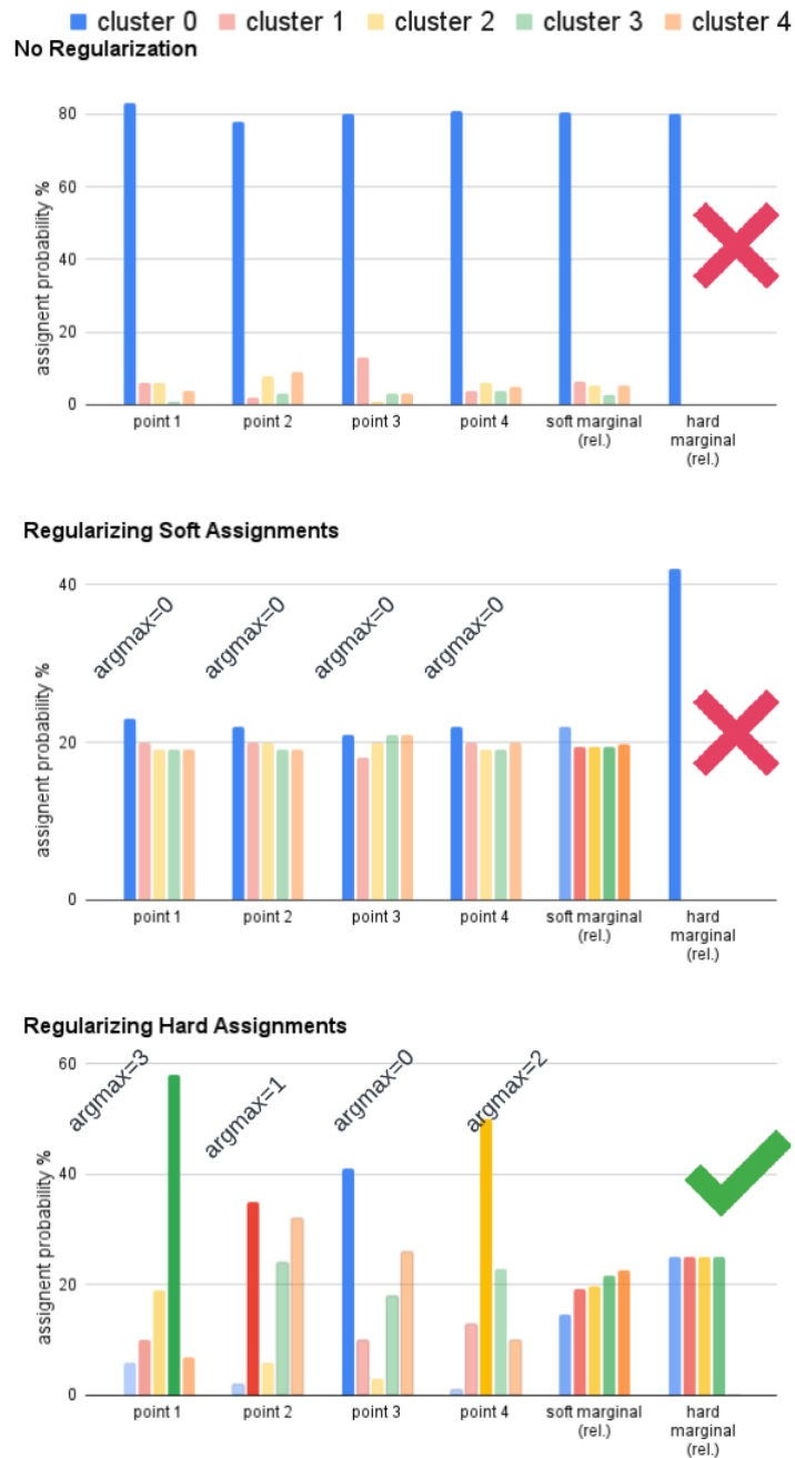
Figure 5.1: Effects of different regularization on the assignments for an idealized batch of size 4, with 5 clusters. Top: with no regularization the model collapses, it places most of the probability mass on the same cluster for each data point. Middle: soft regularization forces the soft marginal assignments to be close to uniform, but still the argmax is the same for every data point, so all points are assigned to the same cluster and the model is also collapsed. Bottom: regularizing the hard assignments causes the argmax to change. It allows the marginal soft assignment probabilities to deviate from uniform, and instead encourages uniformity in the number assigned to each cluster. This model avoids collapse. To make the diagram more readable, marginal assignments are not to scale with each batch assignment, as denoted by (rel.).
