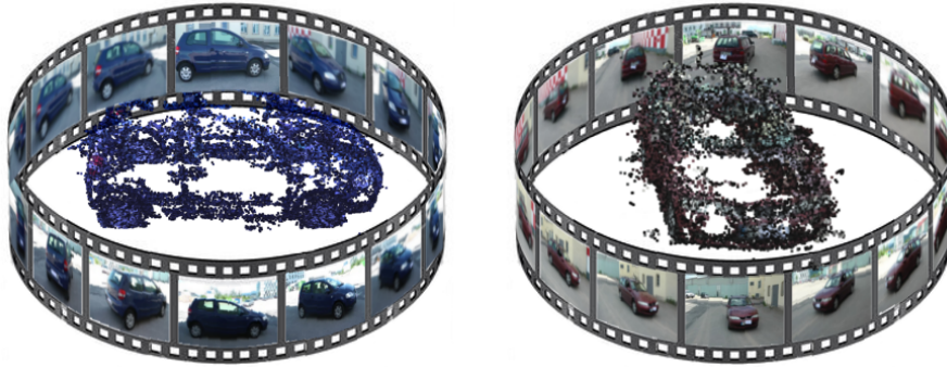
Figure 2.7: Unsupervised viewpoint learning was addressed in [Sedaghat and Brox 2015] where a set of car videos was first reconstructed with an SfM algorithm followed by a collective alignment step utilizing a 3D variant of the HoG descriptor. Image taken from [Sedaghat and Brox 2015].
