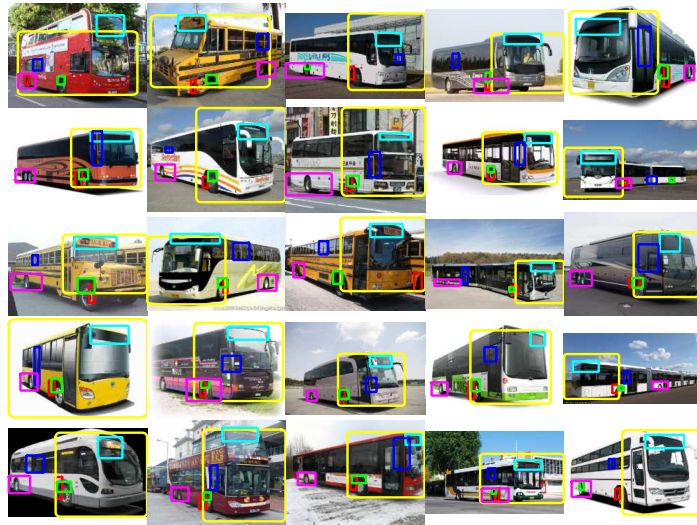
Fig. 6. Visualisation of the bus object class mid-level anchor detectors. Each bounding box corresponds to the max scoring location of an anchor. The locations of corresponding anchors are encoded in the same color across images.
