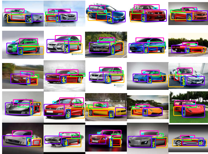
Fig. 5. Visualisation of the car object class mid-level anchor detectors. Each bounding box corresponds to the max scoring location of an anchor. The locations of corresponding anchors are encoded in the same color across images.
