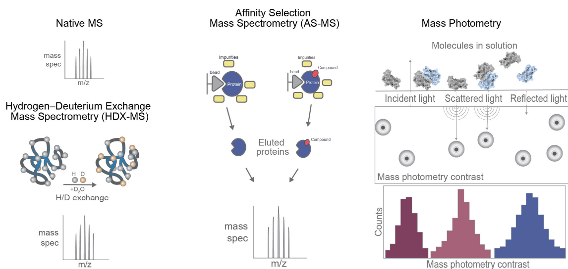
Figure 4. Mass-sensitive sensing platforms expand the range of measurable drug–target interactions beyond simple binary binding. Native MS preserves intact noncovalent assemblies and enables direct determination of binding stoichiometry and higher-order complex formation. HDX-MS reports ligand-induced protection patterns and conformational remodeling by monitoring deuterium incorporation across the protein. AS-MS identifies binders from compound mixtures after target-based enrichment, supporting label-free screening and hit identification. Mass photometry detects individual particles in solution through light-scattering contrast and yields mass distributions for heterogeneous populations and oligomeric states.
