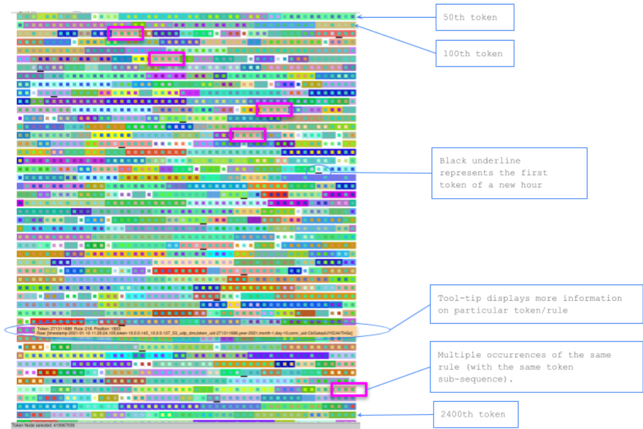
Figure 11: Simple SEQUITUR sequence viewer. Individual event tokens are represented by coloured squares. The sequence of events flows left-to-right, top-to-bottom. Underlaid on the event tokens are coloured rectangles representing recurring sub-sequence patterns extracted by SEQUITUR rules. Tool tips provide detail information for selected event tokens. Adornments relating to absolute timestamps can be added (e.g. which token is nearest to the start of an hour). Note that the purple highlighted borders are manually drawn, to support the narrative in the text.
