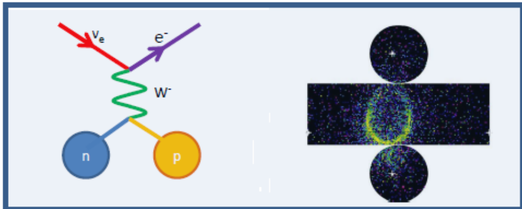
Figure 3.7: A CCQE \nu_e interaction and the image produced by such an interaction in Super-Kamiokande.
