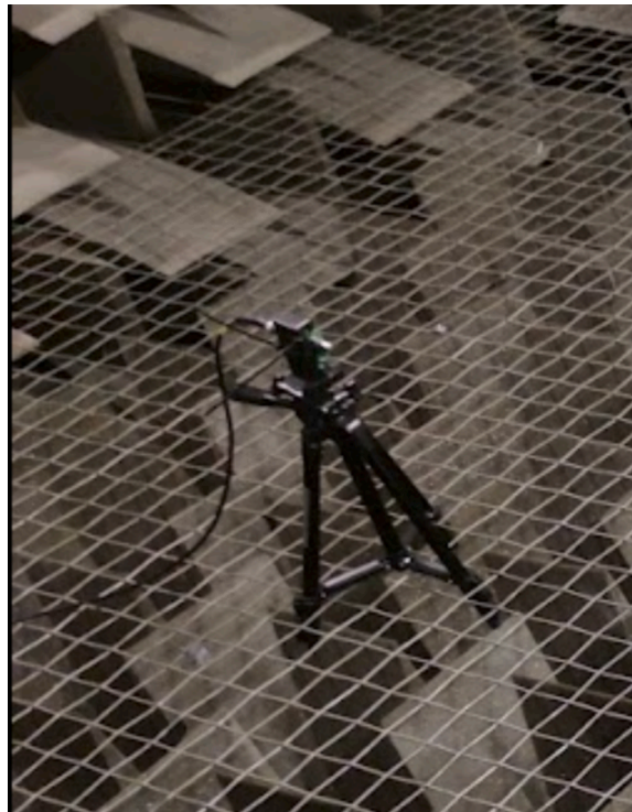
Fig. 6. GRAS 46AE Free-field microphone in anechoic chamber.
