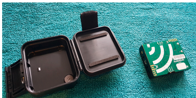
Fig. 1. AudioMoth (right) and its waterproof housing.
