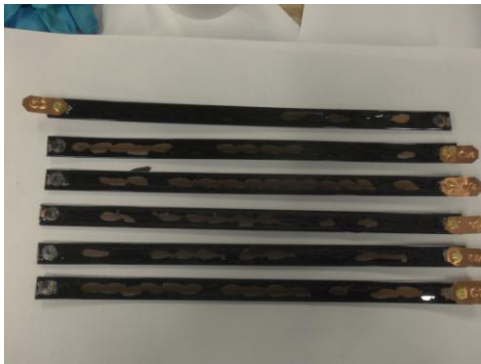
Fig. 15. Aged samples at 275°C after 400hrs.
