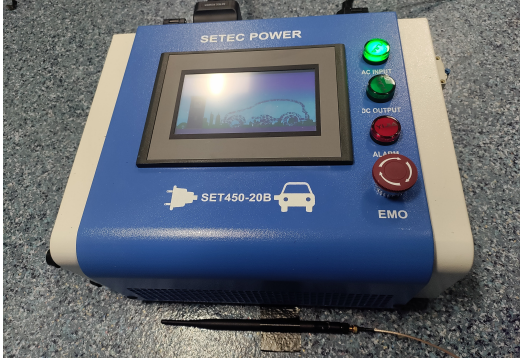
Figure 8: The portable EV charger used in our experiments, as well as the placement of the attacking antenna. The attack is highly effective at 2 W power, despite the metal casing of the charger.
