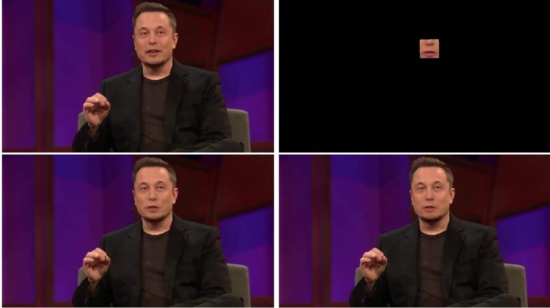
Figure 7.12: Top left: Original still image; Top right: Generated mouth region, aligned with the original (target) face; Bottom left: Generated mouth region, superimposed on the original face. Bottom right: Generated mouth region, blended with the original face.
