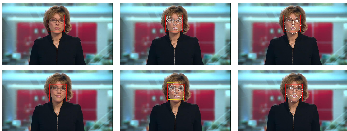
Figure 3.5: Left: Face detections; Middle: KLT features and the tracked bounding box (in yellow); Right: Facial landmarks.
