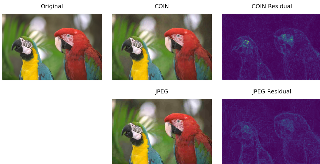
Figure C.9: Comparison between COIN and JPEG on image 23 at 0.3bpp. The PSNRs are 31.08dB and 30.92dB respectively.
