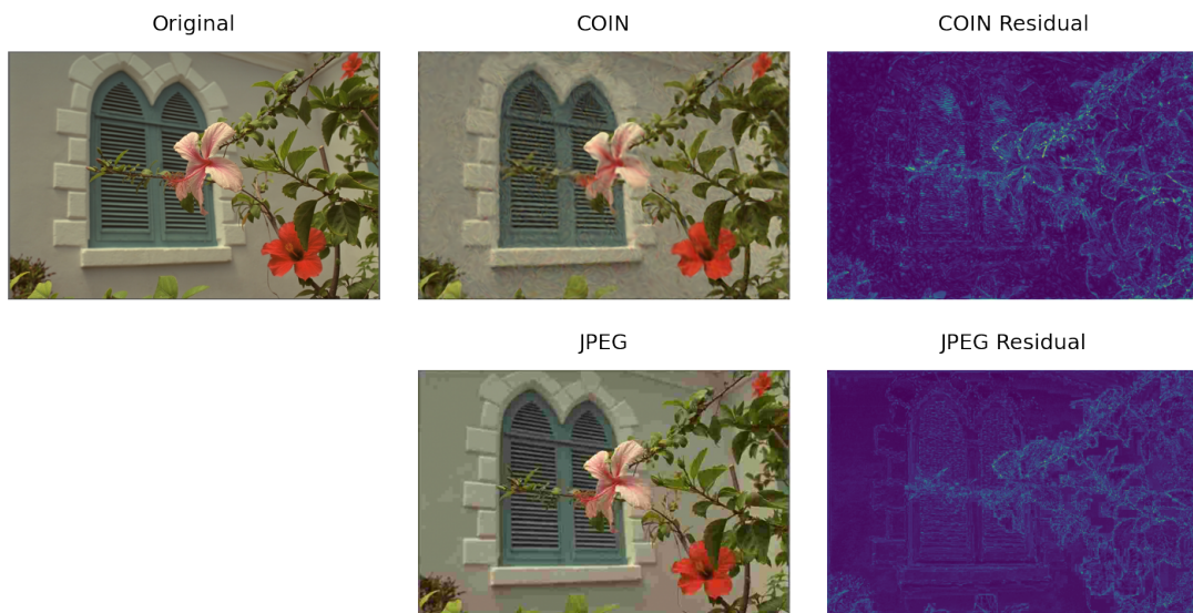
Figure C.5: Comparison between COIN and JPEG on image 7 at 0.3bpp. The PSNRs are 26.92dB and 27.56dB respectively.
