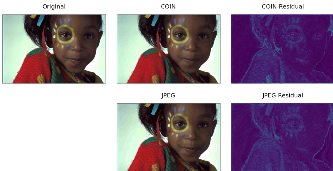
Figure C.7: Comparison between COIN and JPEG on image 15 at 0.3bpp. The PSNRs are 29.31dB and 28.85dB respectively.
