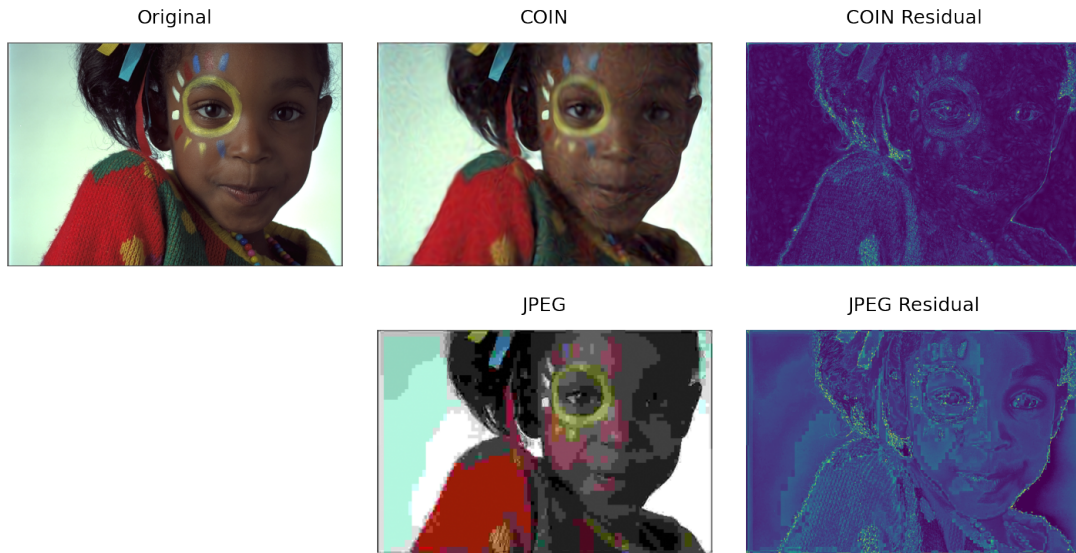
Figure C.6: Comparison between COIN and JPEG on image 15 at 0.15bpp. The PSNRs are 27.35dB and 21.74dB respectively.
