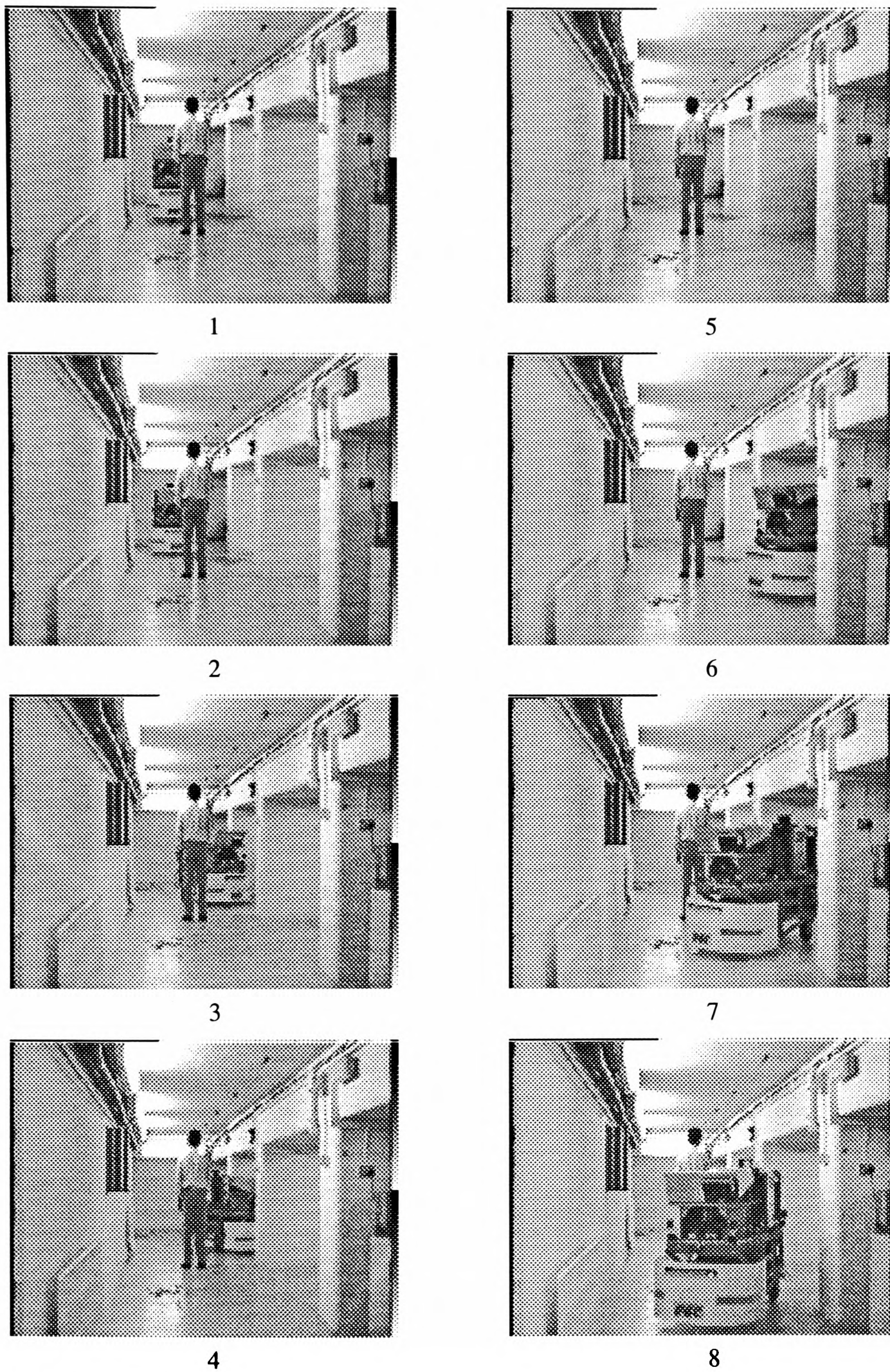
Figure 3.24: The Turtle mobile robot avoids a person who is standing on the way
