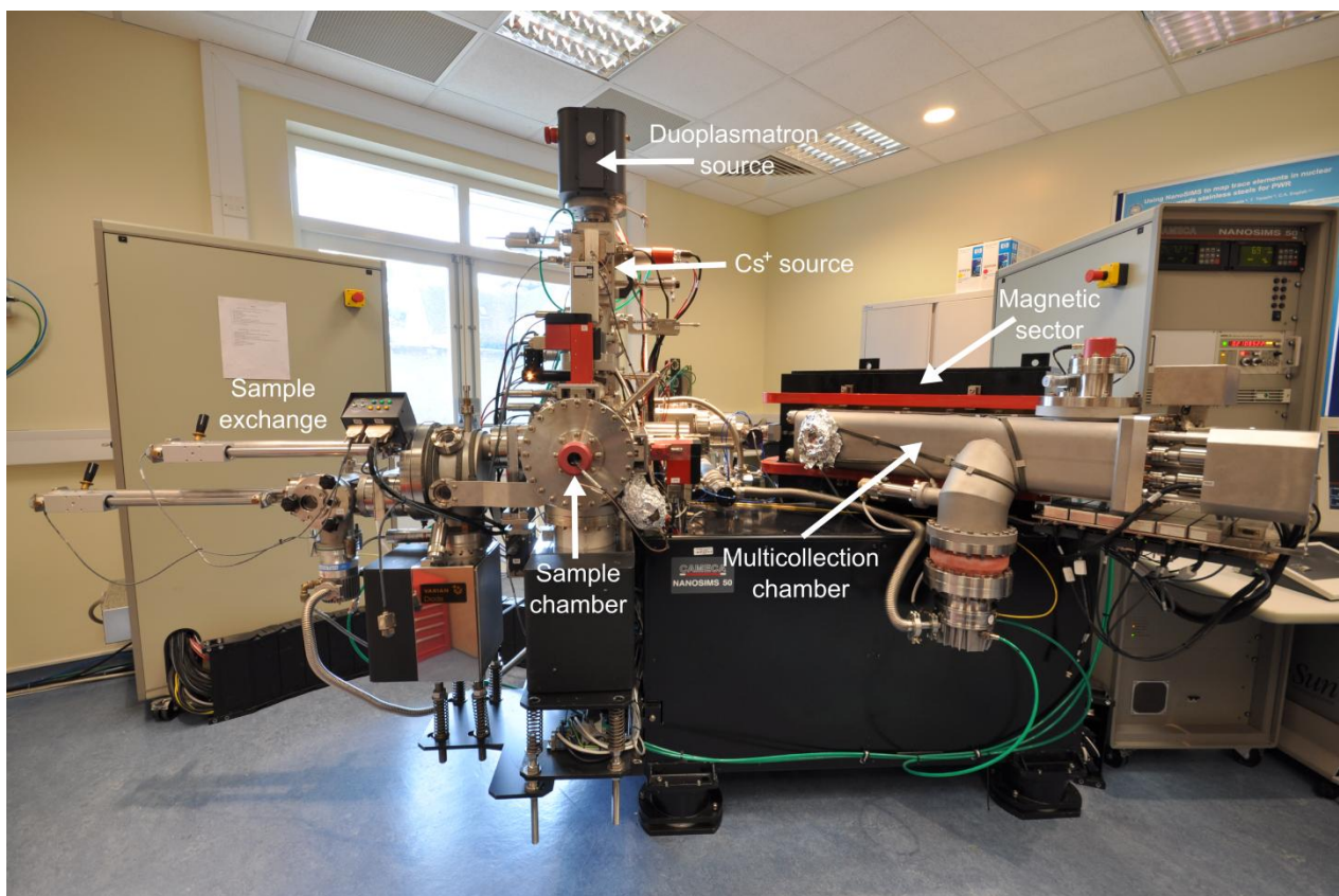
Figure 3.4: The Oxford CAMECA NanoSIMS50 with the key features labelled
