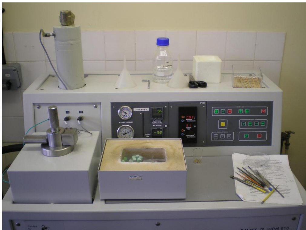
Figure 3.1: The BAL-TEC HPM 010 high pressure freezing machine
