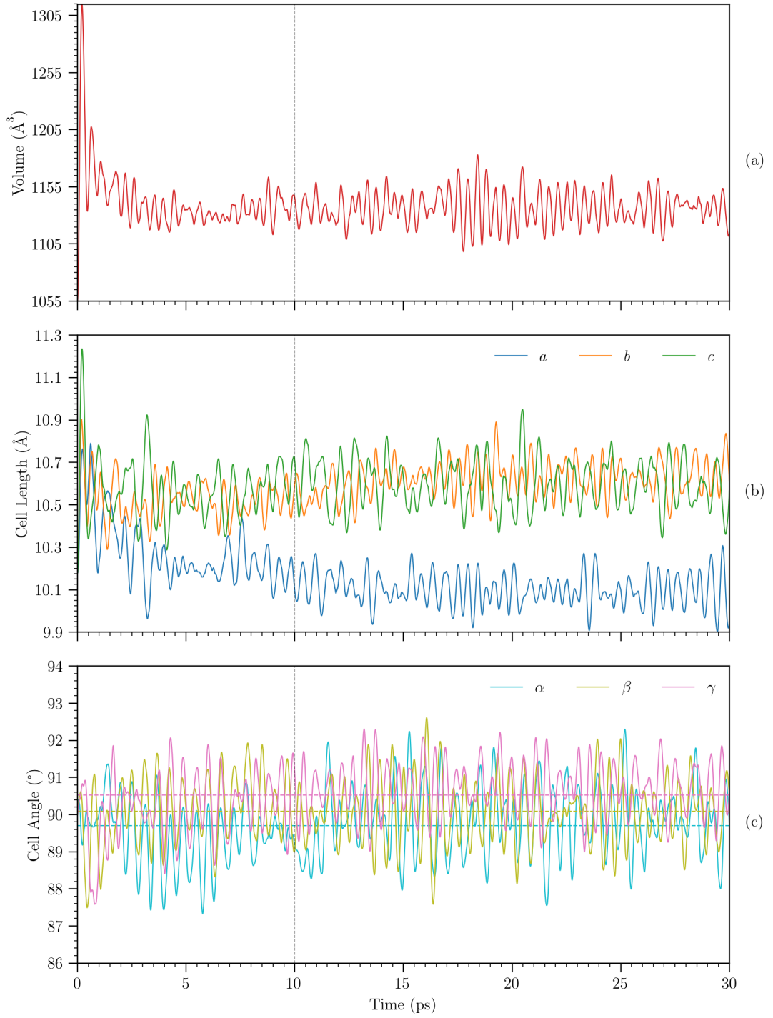
Figure 4.13: \text{Li}_2\text{NH} (a) volume, (b) cell lengths and (c) cell angles at 300 K during the equilibration and complete production run, including the supplementary data collection. The end of the equilibration period is signified by a vertical line. The average angles are plotted in (c) as dashed horizontal lines. In (b) b=c is coincidental and (c) \alpha=\beta=90^\circ while \gamma can vary.
