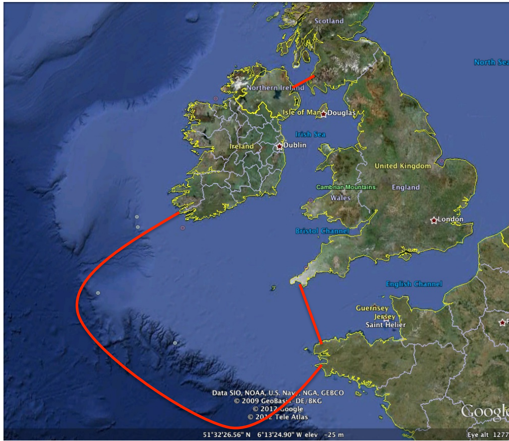
Figure 4.1 – Open boundaries of the computational domain depicted by red lines (Google Earth image, 2012).
