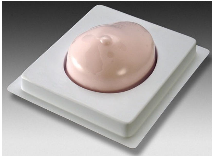
Figure 3- 1 CIRS 059 breast phantom used to obtain reference RF signals for calibration (model CIRS, Virginia, USA).
