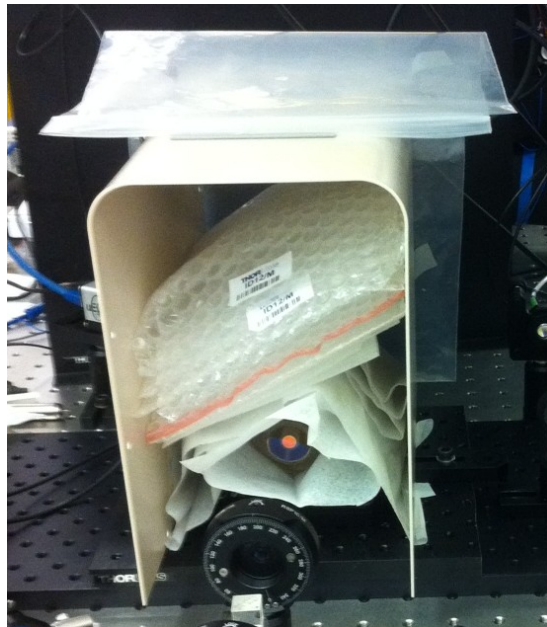
Figure 5.16: Cavity ringdown set-up - showing cavity # 2 mounted on v-blocks on the main experimental table. This set-up was used for initial cavity finesse measurements.
