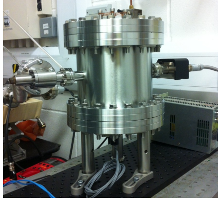
Figure 5.19: All-metal cavity vacuum chamber #2 - The main body is a custom-made DN160CF – DN16CF cross. The top and bottom are custom-made DN160CF flange; one side has the DN160CF knife edge, the other side has an angled wedge for mounting the indium sealed window and M6 bolt holes for attaching the legs. This chamber was designed in-house, and made by LewVac.
