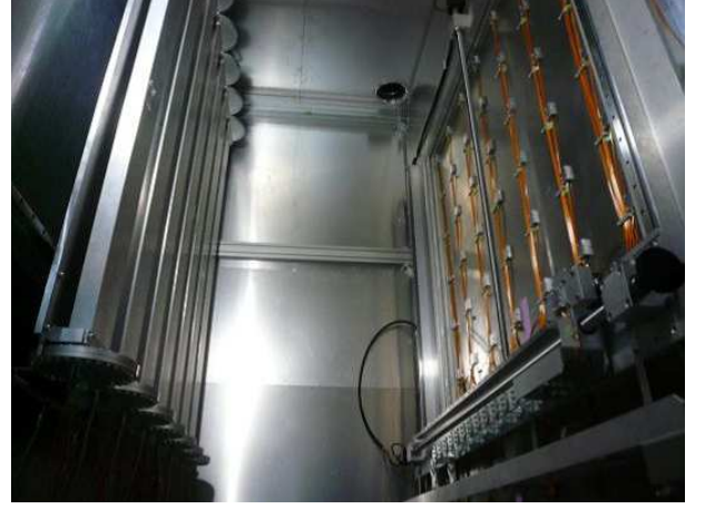
Figure 8: Photograph of the muon monitor inside the support enclosure. The silicon PIN photodiode array is on the right side and the ionization chamber array is on the left side. The muon beam enters from the left side.
