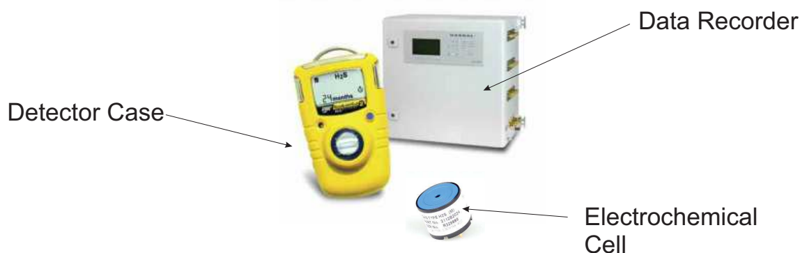
Figure 2.2: Electrochemical gas sensors produced by Honeywell Analytics ( www.honeywell.com ). A electrochemical cell consists of electrodes, membrane and insulate seperators(to keep electrodes away from each other). A detector case has a complete electronic circuit which allows the gas concentration to be read. A data recorder can contineously record the gas concentrations.
