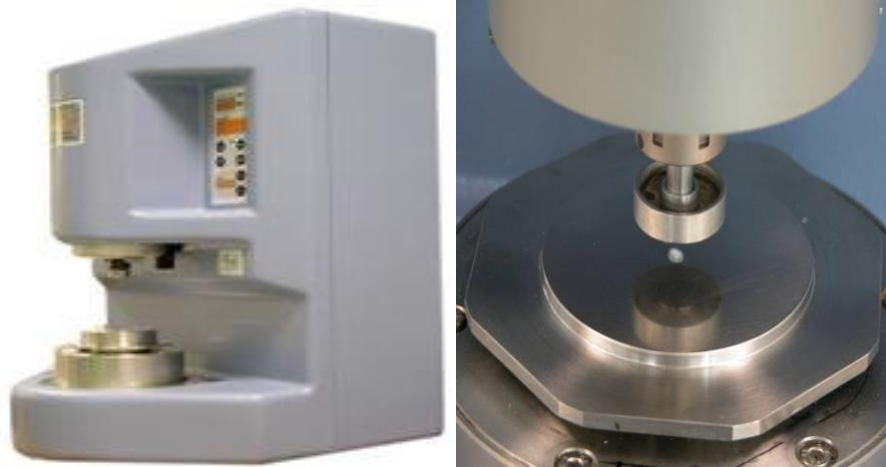
Figure 2-6: Photographs of a rheometer used to test shear properties of rotator cuff tendons. Small 3mm biopsies are tested between two parallel plates.
