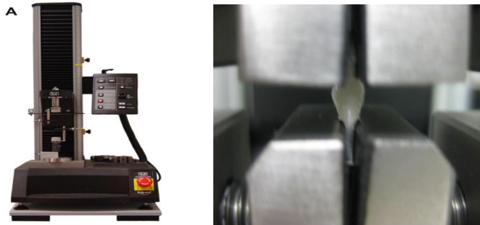
Figure 2-1: A) Photographs of an instron machine used to test tensile properties of rotator cuff tendons. B) Example of a small tendon piece held between 2 large clamps, with only a small testing gauge length.
