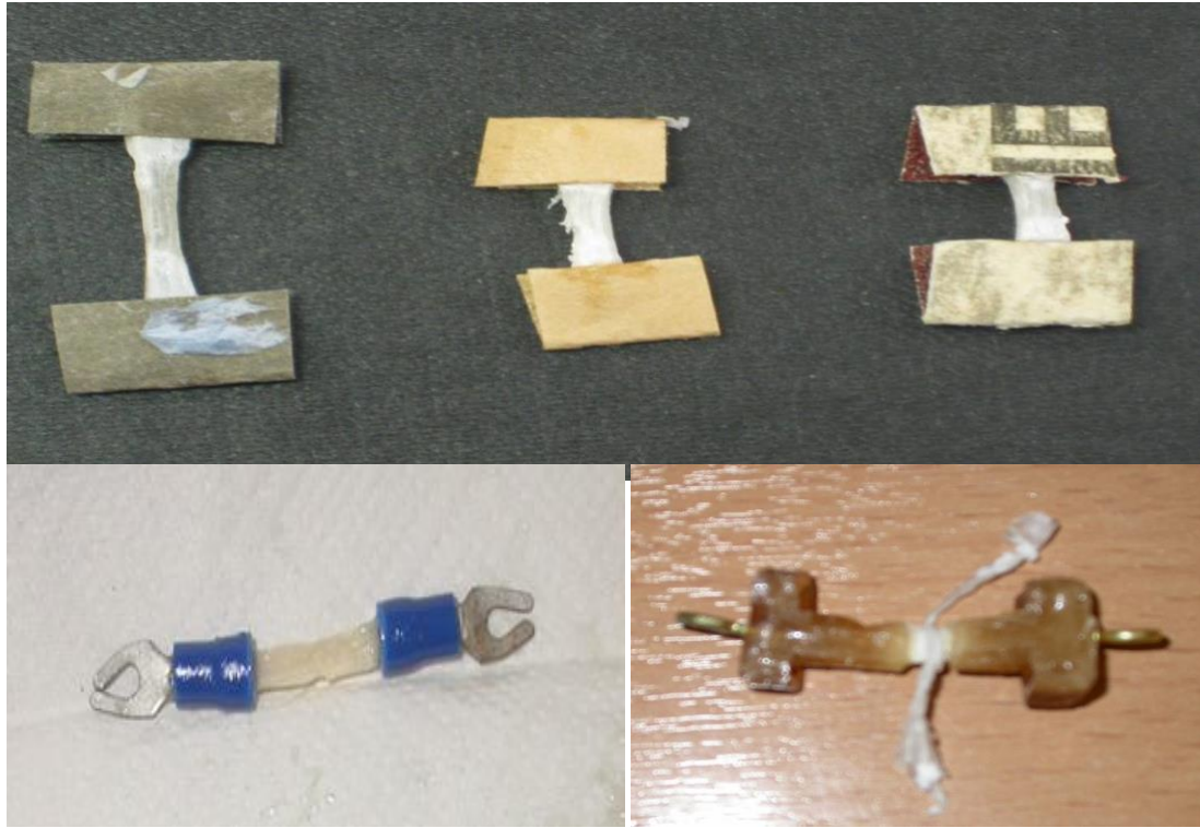
Figure 2-3: Some of the different modalities tried to clamp tendons. A) using sandpaper with differing coarseness B) encased within plastic holders and araldite C) embedded within a collagen matrix
