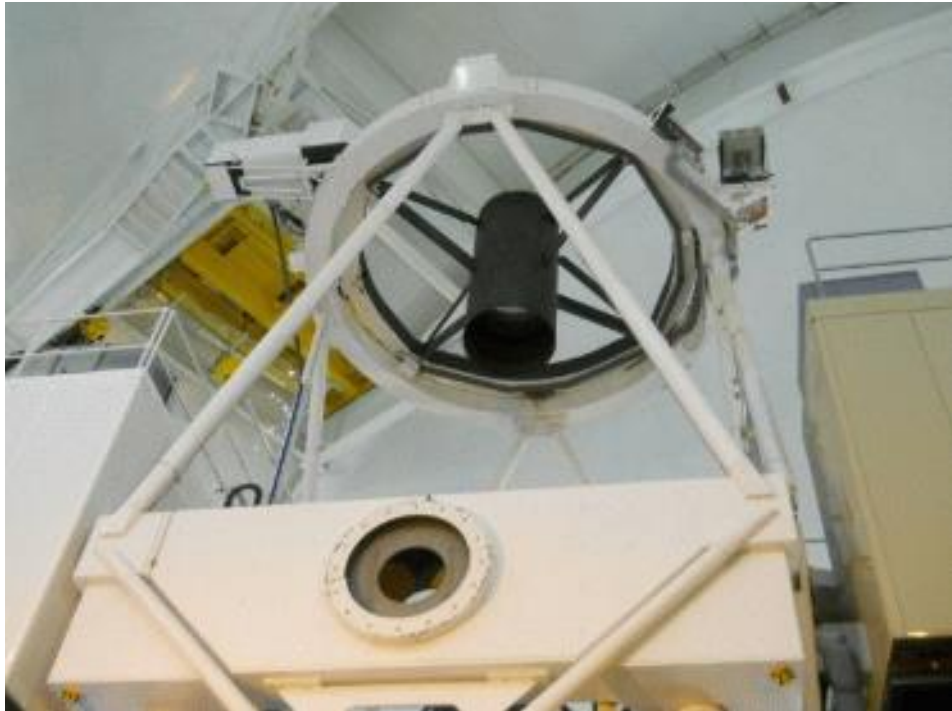
Figure 2 The WHT in the dome. The WEAVE fibre positioner and prime focus corrector will be located at the prime focus of the telescope. The two Nasmyth enclosures, GRACE (left) and GHRIL (right) are shown in the picture. The WEAVE spectrograph will be located within GHRIL.
