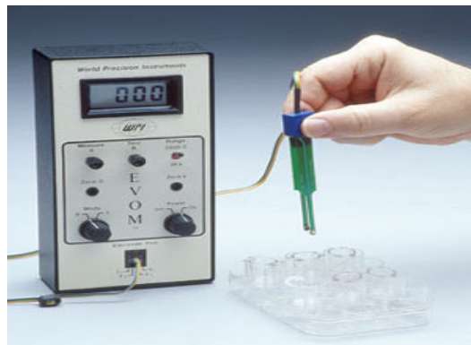
Figure 3.4 Schematic showing a Volt-ohmmeter for measuring transepithelial electrical resistance (TEER) in Transwell ® Inserts. TEER is an electrophysiological measure of in vitro cellular permeability which indirectly assesses formation of tight junctions. TEER was measured on serial days starting from Day 1 post plating until the maximum was reached at which point it was estimated that cells had attained a near normal physiological functioning in vivo .
