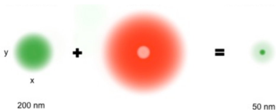
Figure 4.1: Schematic of lasers for STED microscopy. The effective excitation volume is reduced by adding a doughnut-shaped STED laser to de-excite the fluorophores, except those in the centre. This improves the resolution beyond the diffraction limit of light to ~50 nm. From left to right: conventional microscopy excitation volume, STED laser, effective excitation volume in STED mode.
