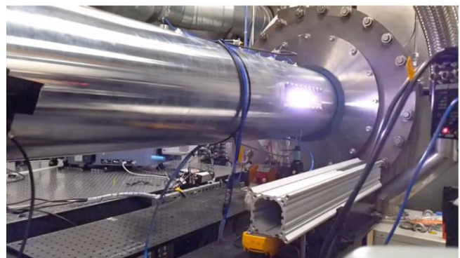
Figure 7: Picture of T6 during air shock layer radiation tests in Aluminium Shock Tube mode.
