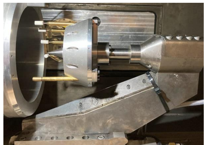
Figure 17: Picture of ring of models for satellite demise testing in T6.
