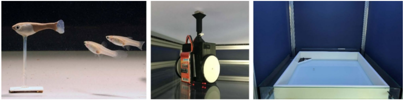
Figure 1. Figure from Maxeiner et al. 23 (CC BY 4.0), showcasing the RoboFish system. Left panel; a 3D-printed fish replica is attached to a magnetic base, which aligns with the robot. Hence the replica can be moved directly by the robot at constant height. Center panel; a wheeled differential-drive robot moves on a transparent platform below the test tank, carrying a neodymium magnet. Right panel; the tank is a quadratic (1 m × 1 m) with a triangular start box used as shelter for the live fish at the beginning of each experiment.
