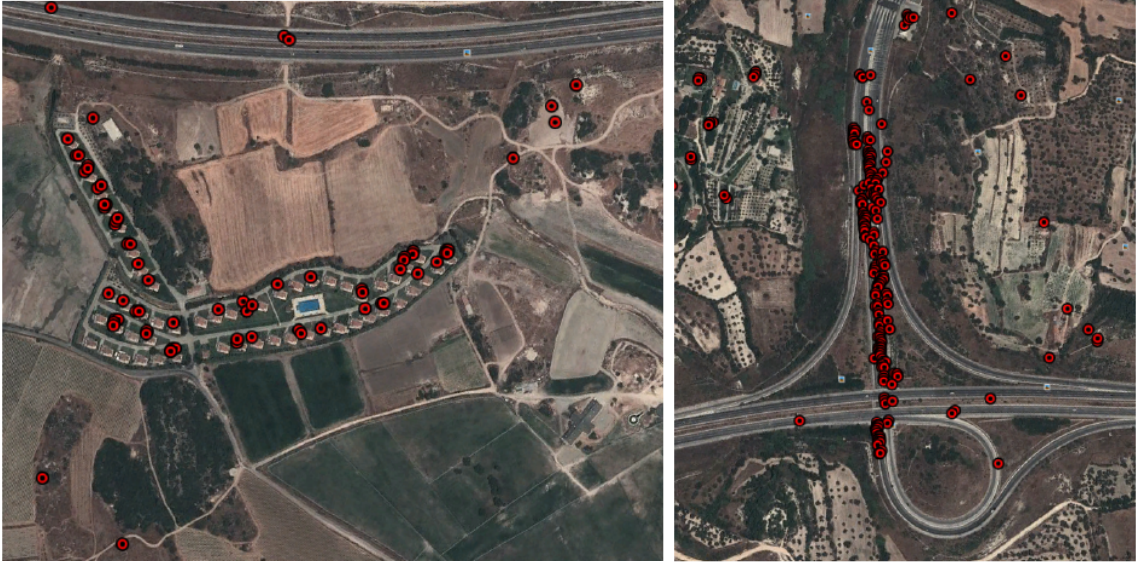
Figure 2.3: Examples of PS selected using a combination of Signal-to-Clutter Ratio and amplitude dispersion in an urban environment using GAMMA. Here the corners of buildings in a housing development and a central reservation barrier along a motorway are the source of PS clusters. This data is taken from track 14 in the region surrounding Izmir in Western Turkey.
