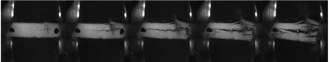
Figure 4.32: Initiation and propagation of damage in a high strain rate experiment
