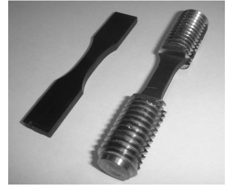
(b) specimen with and without end-caps
