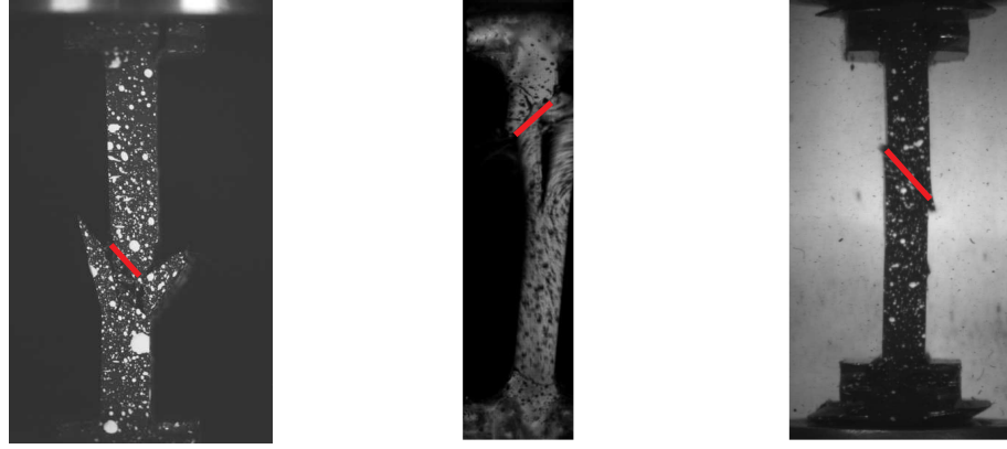
(a) Fracture plane as observed at quasi-static strain rate (b) Fracture plane as observed at medium strain rates (c) Fracture plane as observed at high strain rates
