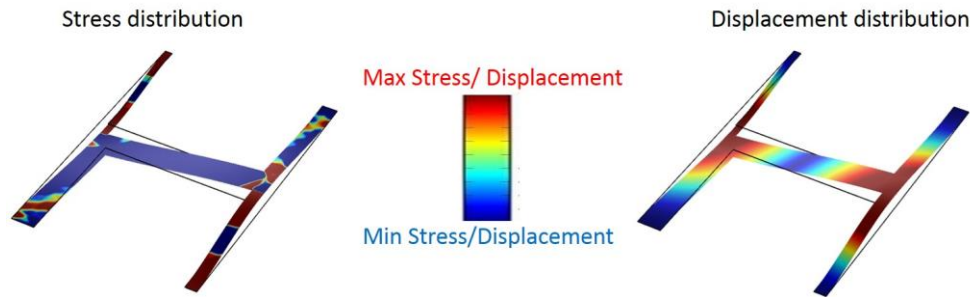
Figure 5. 2 Distribution of the stress (left) and displacement (right) across the beam at the antisymmetric mode of the resonator. Due to asymmetry in the legs of the beam, stress is not distributed uniformly across the two free edges of the resonator and hence amplitude of vibration will be different.
