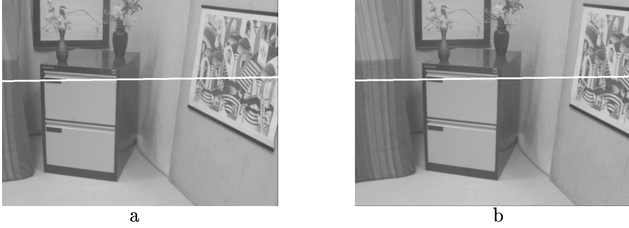
Figure 4. The motion between (a) and (b) is a rotation about the camera centre, with the rotation axis approximately parallel to the image y -axis. The white line is the fixed line \mathbf{l}_r computed from the eigenvectors of \mathbf{H}_\infty .
