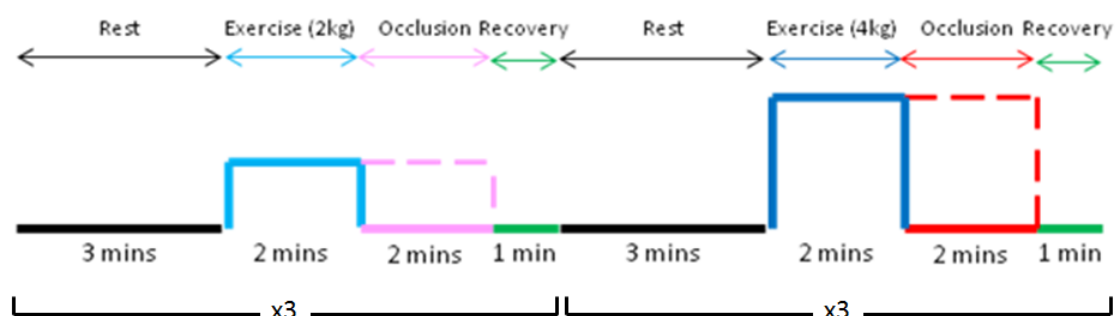
Figure 4.1 – Protocol for increased intensity exercise experiment. The vertical axis represents the level of activity. The solid lines show the actual level of activity of the patient and the dotted lines represent the continued stimulation of the exercise pressor reflex, even though activity has stopped.
