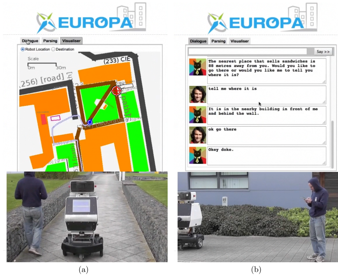
Figure 1.1: A trial of the robot effectively demonstrating the dialogue system, mobile interface and spatial algorithms working together, integrated on a robot platform.
