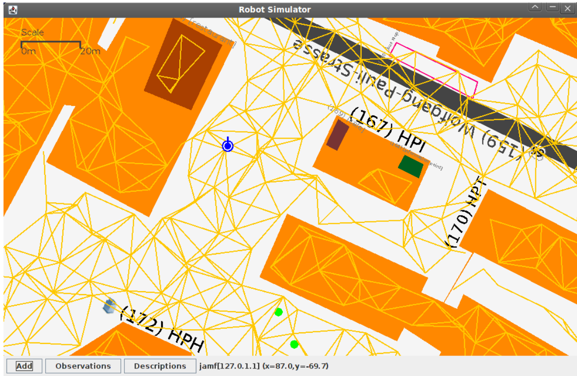
Figure 6.3: A randomly generated graph showing the traversable region of the robot, and allowing routes to be found via A* when the physical robot is offline. Note that due to a designated entrance for the leftmost object, an extra edge is added to the graph to ensure the interior of the building is accessible.
