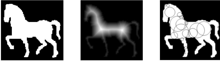
Figure 5.6: (Left) Object instance binary mask; (Middle) Distance transform based representation of the binary mask, (Right) Illustration of the process of reconstruction of the binary mask from its distance transform based representation. This is done by superimposing discs, at every pixel position, of radii equal to the underlying distance values. (Images taken from wolfram.com )
