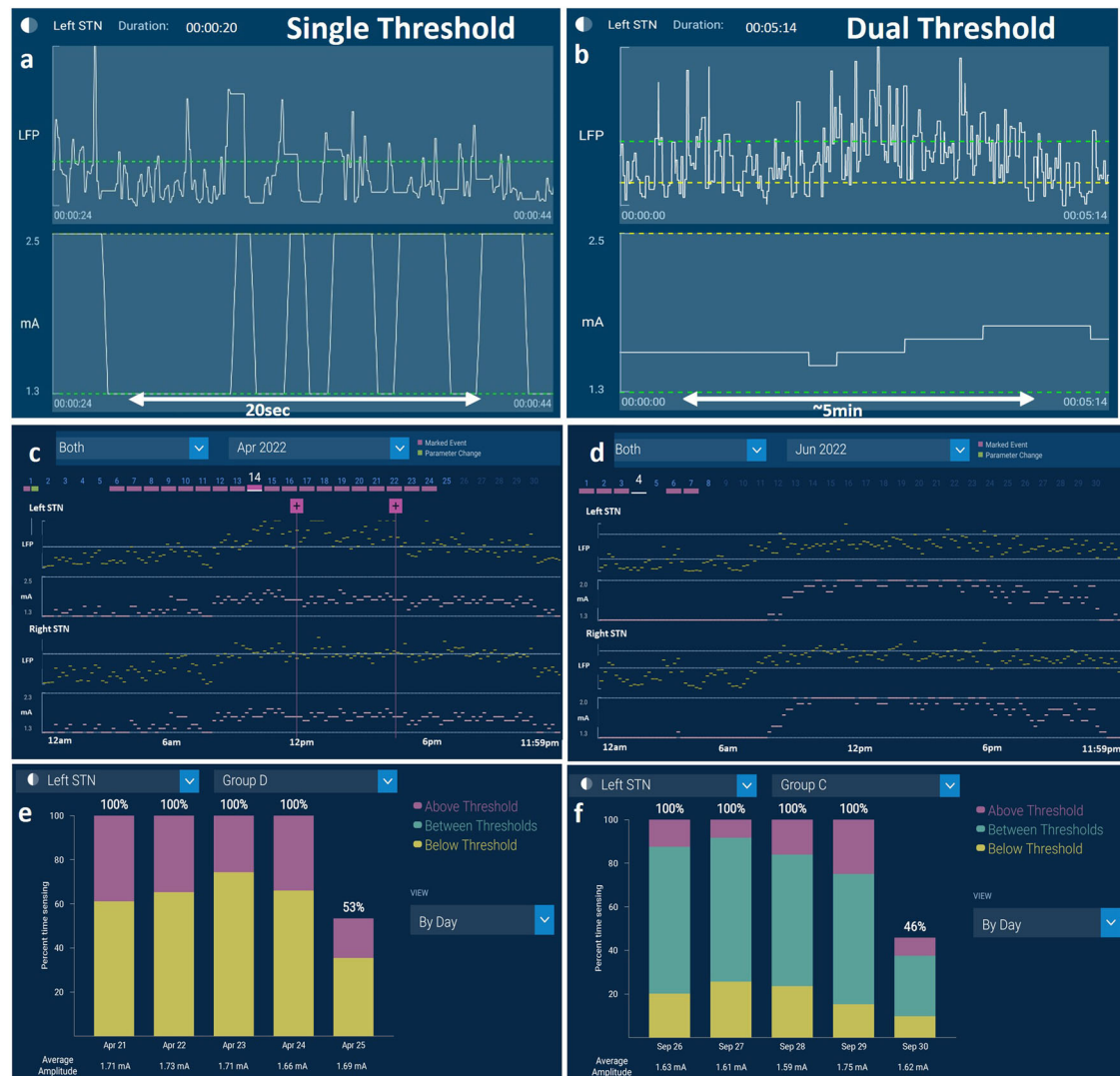
Fig. 3 | Example of LFP signal visualization during aDBS delivery. BrainSense streaming feature enables visualization of stimulation amplitude adjustment during LFP signal fluctuation above or below LFP thresholds for single threshold ( t = 20 s) (a) and dual threshold ( t = 5 min) (b) mode aDBS; BrainSense Timeline feature demonstrating a 24-h interval of LFP signal fluctuation (yellow) and aDBS
